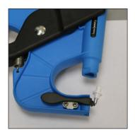
Remove the punch from the applicator and check that sampling has been successful. If not, discard the sample and proceed with a new punch. Remove the used cutter from the applicator by pulling the handles apart. Discard carefully as the cutter is very sharp.
