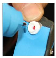
Remove the red plastic clip by pulling it outward. Be careful as the metal cutter above the clip is very sharp. Ensure the applicator is loaded with an unused punch (if the red plunger is visible, the punch is used and should be replaced with one that is unused).
