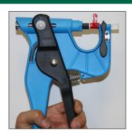
Insert the punch into the applicator. Release the clip to lock punch into the device. Carefully squeeze the applicator handles together, guiding the punch tip into place if necessary. When the gun bolt rests flush against the red plastic clip, release the handle.
